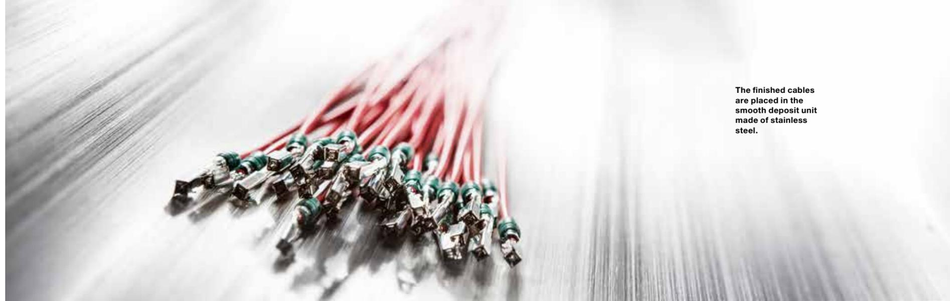
The finished cables are placed in the smooth deposit unit made of stainless steel.
