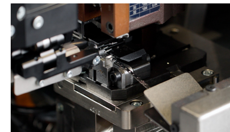
Symetrical crimping with the CP 150
