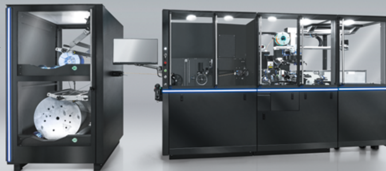
▲ Optima 600 configuration with 2-spool dereeler and WCT, WSI, WEL modules
