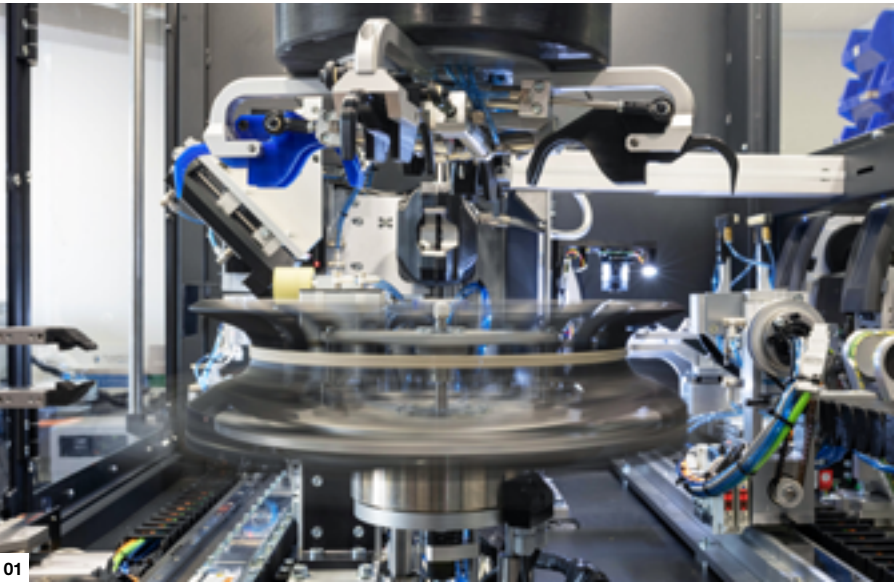
02 Two independent and fully programmable grippers handle wire extremities.
