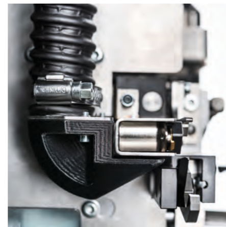
Optional suction unit for stripping remnants
