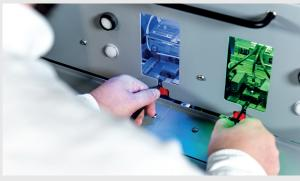
With the function manual wire insertion, it is possible to insert the cables one sided or both sided. Additionally, wires can be inserted already pre-assembled on one side.
