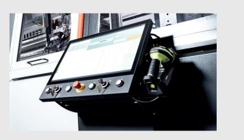
Optionally a movable and tiltable control unit can be installed in front of the machine which can be moved manually over the entire process level.
