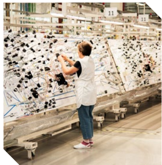
Worker at a wire set routing board in a customer's factory. Due to the highly individual nature of the product, the assembly of wire harnesses is still manual work today, but modern automation technologies could change this in the near future.
