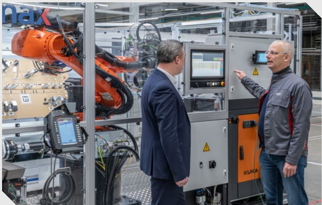
Prototype implementation of a complete system for manufacturing and assembling a center console wiring harness at the AUDI AG plant in Ingolstadt, Germany (photo: AUDI AG).
