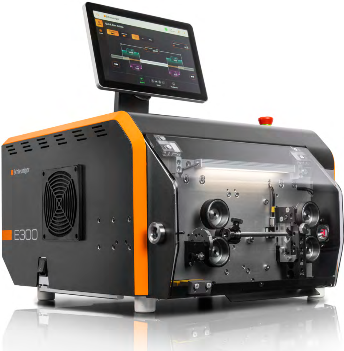
01 | 02 Different feed belts and coatings of the rollers ensure optimum transport of the cables. The contact pressure on the feeding unit is programmable. The E300 is equipped with a two-in-one quick-change feeding unit suitable for roller drives, including a short piece kit for the processing of short cables. 03 The E300 cut & strip machine can be combined with many peripherals to form an automatic processing line. Existing Schleuniger peripherals are compatible. 04 Minimal training effort and extremely short commissioning thanks to S.Drive software.
