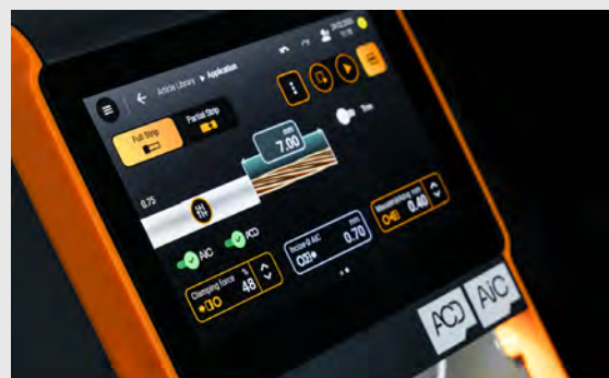
▲ A glance at the display of the Schleuniger Strip Series B300 with Adaptive Conductor Detection (ACD) and Adaptive Incision Control (AIC) enabled.
