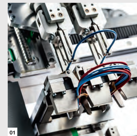
01 The bundler sorts and binds the batches in a single process step. 02 Parallel processing set with 3 shuttles for top performance.
