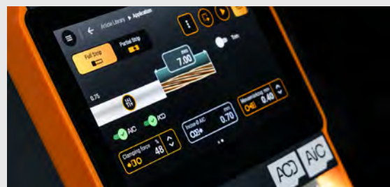
▲ A glance at the display of the Schleuniger Strip Series B300 with Adaptive Conductor Detection (ACD) and Adaptive Incision Control (AIC) enabled.
