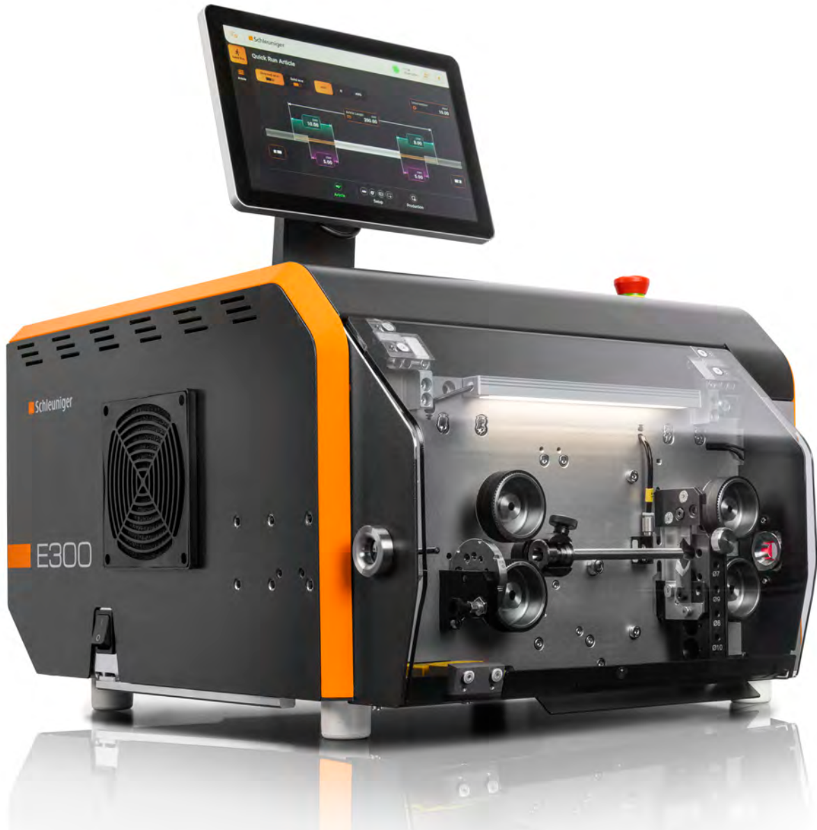
01 | 02 Different feed belts and coatings of the rollers ensure optimum transport of the cables. The contact pressure on the feeding unit is programmable. The E300 is equipped with a two-in-one quick-change feeding unit suitable for roller drives, including a short piece kit for the processing of short cables.
